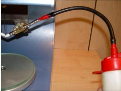
7. Add three or four drops of oil in the holding devices **A2** and wait at least two minutes before starting to use the device to perform a test.
