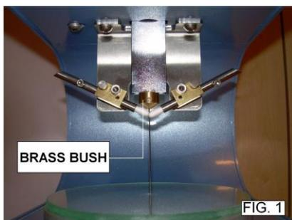
3. Insert plugs **A4** in the corresponding holding devices **A2** and fix them as described in Section 5 Plug Replacement.
