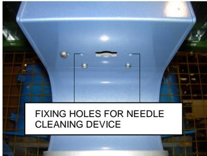
1. Place the cleaning device on the Vicat machine so that the fixing holes on the appliance are centered with those on the Vicat.
