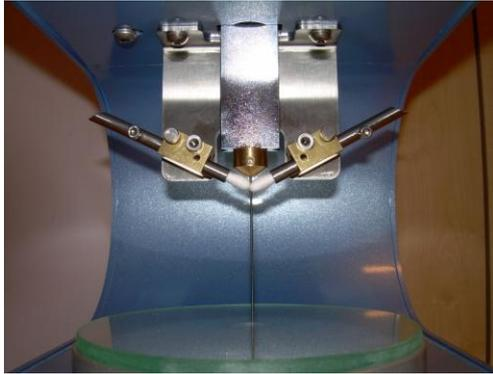
4. Push button **A3** again, insert the holding devices so that they adhere perfectly to the needle of the probe (as shown in the previous section), then release the button.
