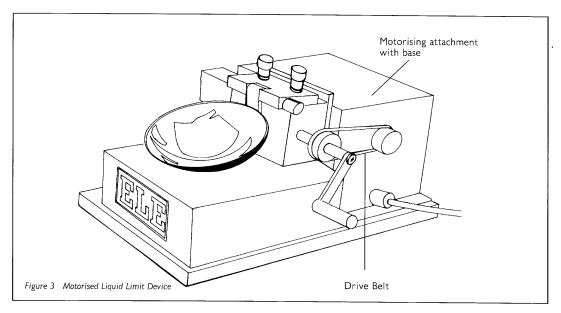
2.2.2 The liquid limit device incorporates a drive assembly with drive and follower pulleys, the latter fitted on the cam shaft of the liquid limit device. A blow counter is included in the motorised version.
