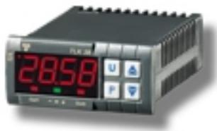
A TLK38 digital cut out protects the contents of your incubator by allowing you to program over & under temperature safety cut out set points. When the chamber temperature goes out of limits, an audible alarm and visible red neon will bring to your attention any problems. Reset buttons are provided below the cut out for you to manually reset the out-of-limit system.
