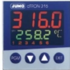
The **yellow 3** on the temperature controller shows when heat is being supplied. The **yellow 5** shows when cooling is being supplied.
