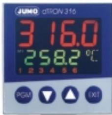
The temperature is accurately controlled by a Jumo dTRON 316 microprocessor temperature controller. The controller uses the signal from a PT100 sensor located in the chamber to control the current supplied to the heaters. The temperature can be easily adjusted. See Section 3 for details.
