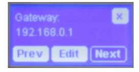
Power cycle the DSU off for 10 seconds and then back on. Confirm the IP Address settings have been correctly entered and stored.
