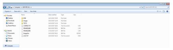
In order to update the firmware file, take a copy of the existing file and save it to another location. Copy and paste the updated firmware file into the root directory of the DSU, selecting "Copy and Replace" when prompted.
