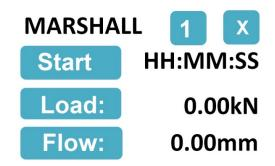
Once the test has been started data acquisition commences once a 1kN load is seen. Ten samples are recorded every second.
