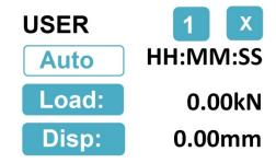
The data acquisition rate occurs at a rate defined by the sample length and applicable to both ASTM and BS standards. If the frame used was a Multiplex, then the 'Start' button will appear as 'Auto' and the control of the test start will be entirely from the Multiplex frame.
