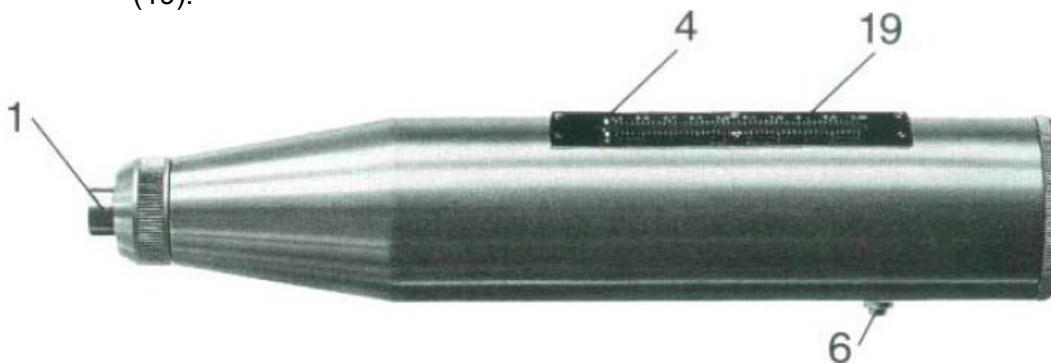
Figure 2.4 Reading the test result from the scale (19)
