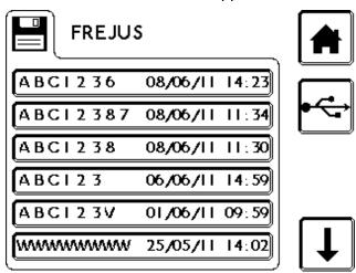
Pressing the USB icon activates the USB link. The unit should appear as a simple memory device with no special device driver files being needed. The screen should appear as shown. **Note:** No monitoring of the sample's load occurs whilst in this mode.
