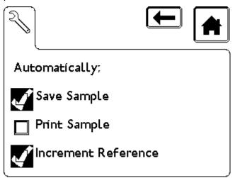
In this screen you can set the system to save all sample test details, print all test reports (after each test) and apply an increment to the selected test reference. Pressing the box will apply a tick.
