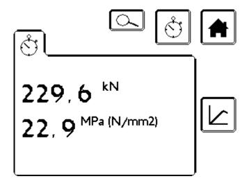
To prepare the ADR for the next sample, press the icon to return to the Test Screen. Otherwise the test result could be examined further by touching the Magnifier icon, where the screen will then switch to show the sample failure details and will be of the form –
