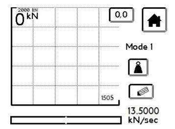
The Pace Error Bar display shows the difference between the required rate and the rate achieved by the operator. The default range of the error bar is normally ±5% of the set rate.
