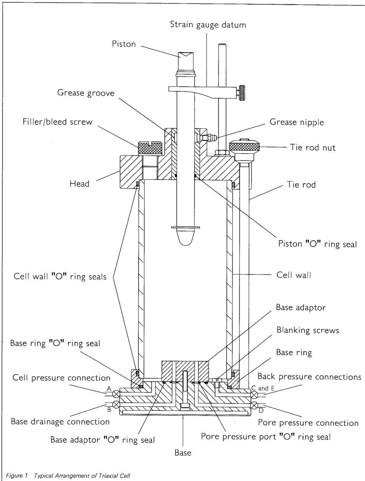
Figure 1 Typical Arrangement of Triaxial Cell
