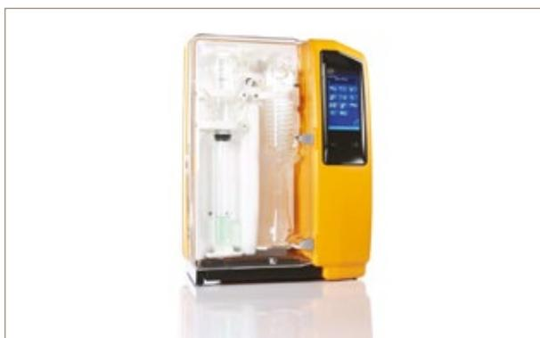
This distillation unit is fully automatic with full microprocessor control. The operator has only to insert the digestion tube and the distillate receiver vessel. The control display is a back-lit LCD with 2 x 16 character lines. Information is entered via the touch sensitive keypad which has numerical characters for entering distillation program parameters, and manual function keys to activate the chemical addition pumps and for programming.
