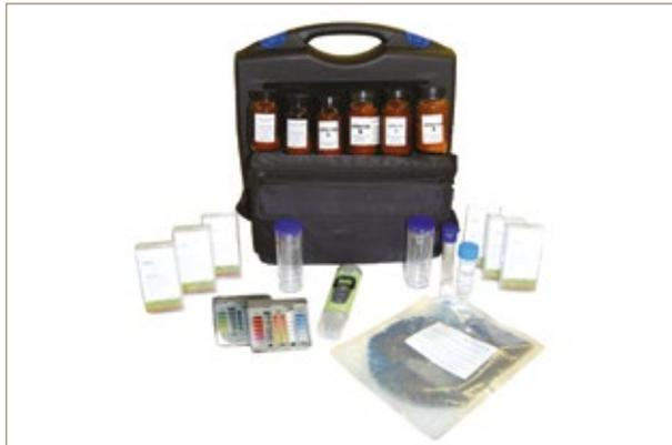
This test kit measures soil pH, conductivity, N/P/K, magnesium and calcium using simple visual test methods. It is durable, designed for field use and includes:
