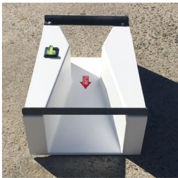
Throat width 100 mm, for measuring flows in the range 0 to 15 litres/second.
