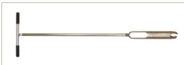
One piece model, length 1.25 metres. This auger is used in hard stiff soils above and below ground water level. It is also satisfactory in most fine gravel soils. 2 cutting head sizes available.
