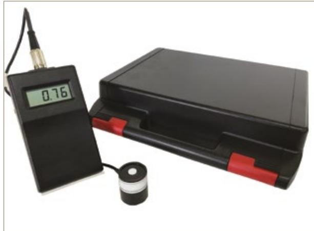
General measurement for human activities. The visible light is that part of the wavelength spectrum received by the human eye. The peak sensitivity is 555 nm for the adapted eye but with 'dark adaption' a peak response is 507 nm. The ranges allow for readings between 0 to 200 K Lux. The sensor has a cosine-corrected head, and the FET input circuitry of the cc measuring and display unit preserves linearity. The unit also incorporates dual slope integration with "auto zero" for A/D conversion.
