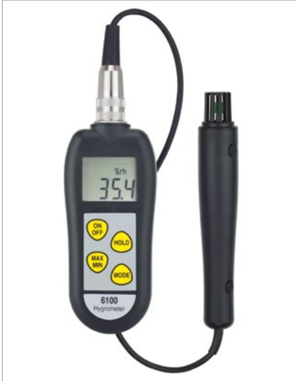
Remote or integral % RH and temperature probe. Displays maximum/minimum humidity or temperature. Optional backlit display. The therma-hygrometer is an easy to use, relative humidity and air temperature measuring instrument. The units measure % RH over the range of 0% to 100% RH with a resolution of 0.1% RH and temperature over the range of -20°C to 70°C with a resolution of 0.1°C. It incorporates a custom LCD, displaying % RH, °C/°F, dew point indication, maximum/minimum and hold.
