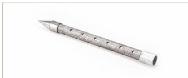
Comprising a porous plastic element. 19 mm diameter x 300 mm long, in a perforated steel tube with hardened steel driving point. Terminates in a 3/4 inch BSP pocket.
