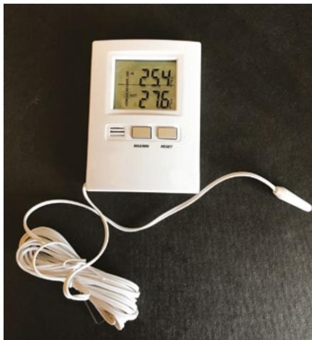
This digital thermometer can be wall-mounted or free standing to display the ambient temperature. A plug-in probe with 3 metres of cable can be used to obtain the temperature in another area or from outside. The instrument has a memory to recall the maximum and minimum inside and outside temperatures since the last reset. Switchable between °C and °F.
