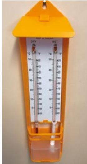
The wet and dry bulb hygrometer is designed for general use and consists of two undivided thermometers mounted on a printed plastic scale. Between the thermometers is a unique slide pointer which allows relative humidity to be easily read. The scale is housed in a plastic case which also holds a reservoir with anti-frost device.
