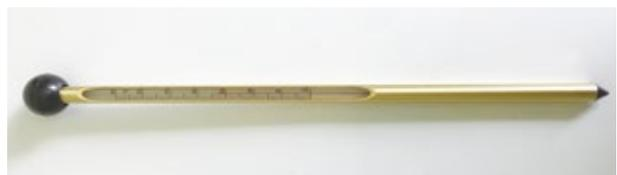
Range -10°C to +60°C, in a rugged brass case with stem graduated at 5, 10, 15, 20, 30 cm to enable measurement at various depths. Ideal for use in education.
