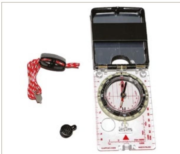
With inclinometer. A folding pocket instrument with sighting mirror in the lid. Used for defining map locations and measuring geological equipment.
