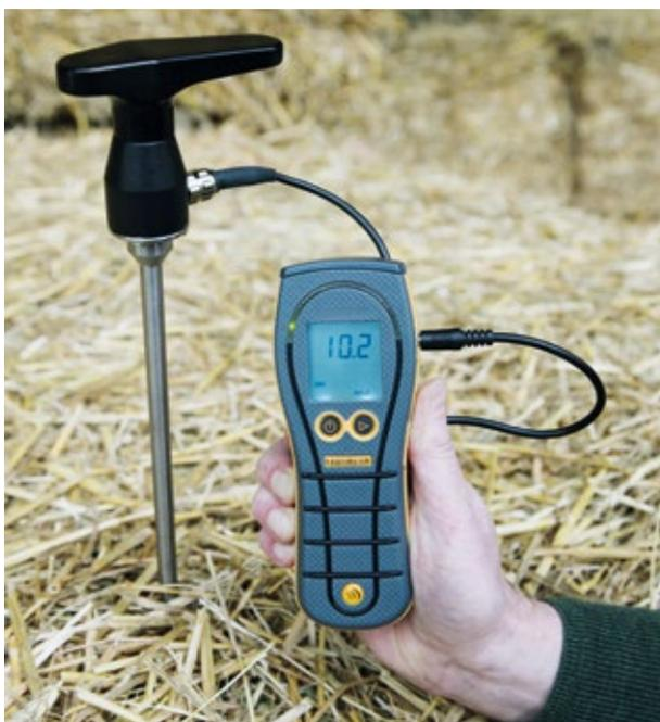
This lightweight hand-held instrument can be used for the rapid moisture measurement of baled hay or straw. The strong Stainless Steel probe is inserted into the bale and the test button pressed. The result is shown instantly on the clear analogue display. A separate button can be used to check the calibration and battery voltage.
