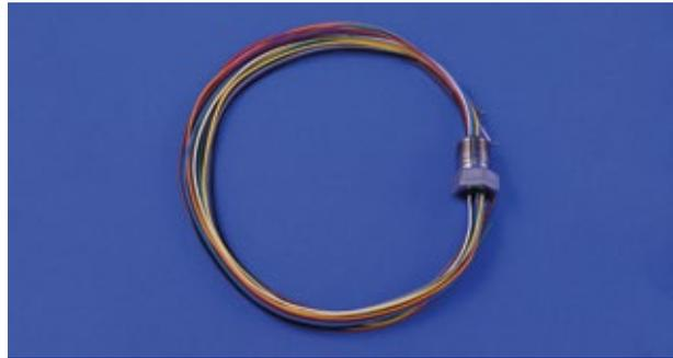
This Stainless Steel 1/4 NPT fitting leads through 10 electrical wires (26 AWG), connected to the fitting with epoxy seal. Handles up to 300 PSI.
