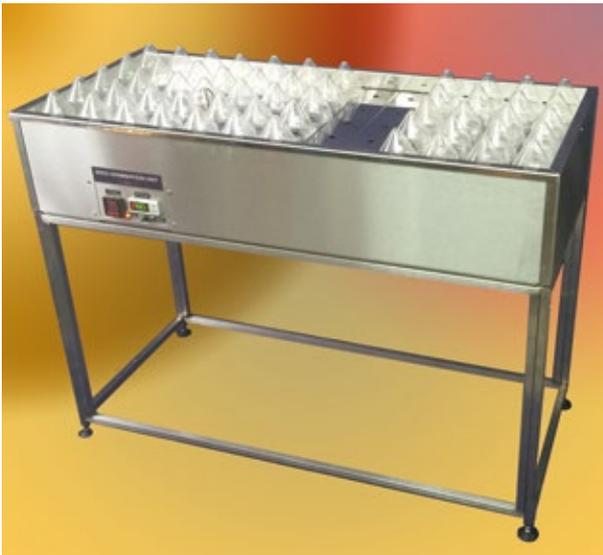
The Jacobsen Seed Testing Bath provides the conditions specific for seed testing according to the regulations of the International Seed Testing Association.
