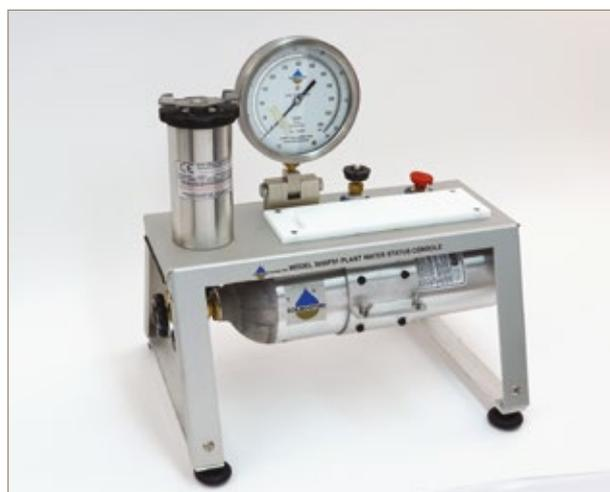
The Plant Water Status Console is supplied with a compressed gas cylinder and connected to a pressure regulator for field operation. The pressure regulator has been set at the factory for the maximum operation pressure of the unit which, for standard units, is 600 psi.
