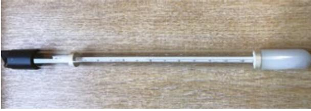
Temperature recordings are made by lowering the thermometer down a tube with a rope or chain. The thermometer bulb is encased in wax to allow a slow change of temperature to be recorded and when the instrument is recovered retaining the reading.
