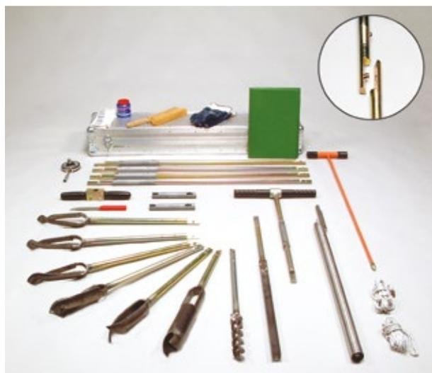
For augering all types of soil above and below the water table to a depth of 5 or 7 metres. Supplied complete in an aluminium transport case with padlock.
