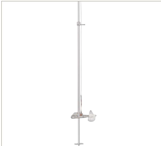
Consisting of current meter, revolution counter, wading rods, base and knob, 3 metre wading cable.
