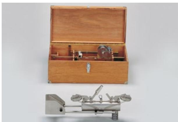
This sampler is designed to be used in a flowing river or stream at any desired depth to 25 metres. The design is such that the open ends through which the water flows can be simultaneously closed, thus retaining the 1250 ml sample which may then be raised to the surface. The accessories include a hand winch, 25 metres of steel wire and a depth meter. The complete set is contained in a wooden transport case with padlock.
