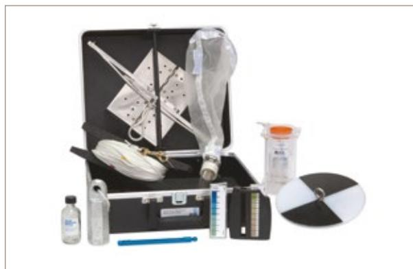
With colour scale, water sampling bottle, plankton net, bottom sampling dredge, sounding lead and calibrated line, 20 metres long marked at 1 and 5 metre intervals, armoured thermometer and Secchi disc (for turbidity check).
