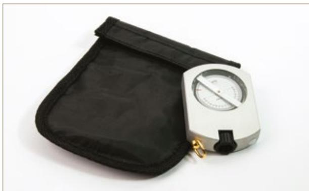
A hand-held precision instrument for determining heights, slopes and vertical angles. The direct sighting device has the peak scale reading visible through the eye piece. Percentage and degree scales permit quick calculation of object heights using a known base line distance. Used by foresters, geologists and surveyors throughout the world.
