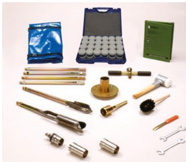
This kit contains the necessary items to sample above and below the water table and comprises the handle and beating head, Edelman auger, a Riverside auger, a closed ring auger and spare cutting shoe, a hammering head and guide cylinder for the rings, a nylon headed hammer, 3 extension rods 500 mm long, 24 numbered sample rings with end caps in an aluminium case, a bent spatula, brush and a carrying bag for all the equipment.
