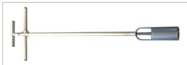
One piece model with 80 mm diameter cutting head. Sample length 150 mm.
