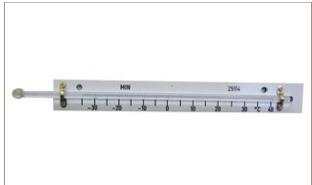
Mounted on plastic scale to match maximum thermometer. Specification as maximum thermometer but recording minimum temperature since last reset, in the range of -35°C to +40°C x 0.5°C.
