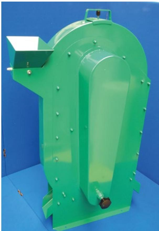
This machine is suitable for pre-cleaning a large number of agricultural products including hulled rice and coffee, wheat, barley and vegetable seeds, by removing light extraneous material such as shrivelled seed, chaff and leaf. Heavy particles including metal and stones can also be eliminated. It consists of an aspirated column with an adjustable flow rate, expansion chamber, air-return ducts and motor driven fan. The fan can easily be removed for cleaning. The unit is bench mounted.
