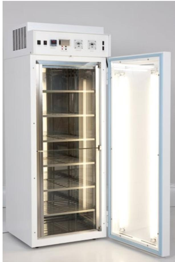
This robust germination unit is constructed in white polyester powder-coated steel, for a smooth, tough, easy-to-clean finish. The plastic coated wire mesh shelves are fully adjustable with 32 shelf positions at 29 mm centres. The dual temperature controller and thermistor system enable two temperatures to be set to correspond with "day" and "night" environments. An adjustable over-temperature safety cut-out protects the contents from accidental overheating.
