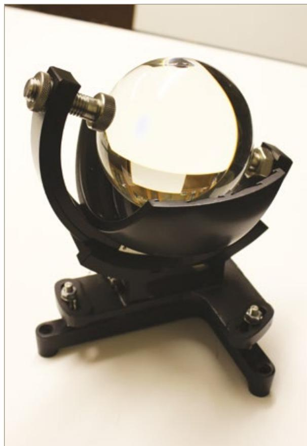
This instrument is used to record the duration of sunshine each day. The sun's rays are focused by a precision glass sphere onto a curved card. The intense heat burns a trace on the card. As the sun moves across the sky, so does the position of the spot across the card. If the sun is obscured by cloud then no trace is made. At the end of the day, the length, less gaps, is proportional to the duration of sunshine.
