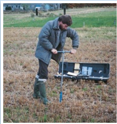
1) Auger and prepare hole
