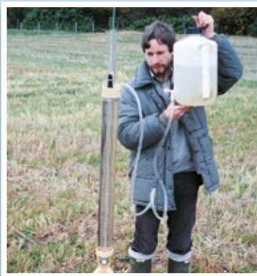
2) Install Permeameter and fill with water
