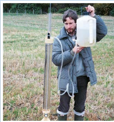
2) Install Permeameter and fill with water
