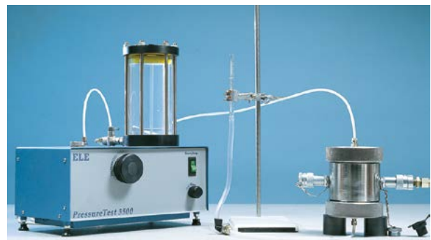
Permeability Test with Pressure Test 3500 Pressure System.
