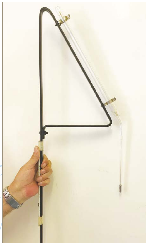
Metal support frame for use with Earth Thermometers.
