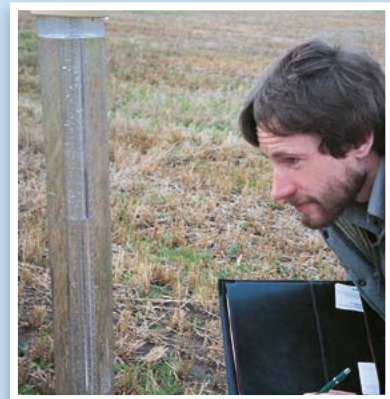
3) Record changing water level and calculate results
