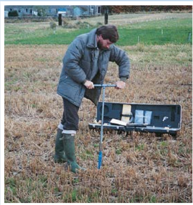
1) Auger and prepare hole
