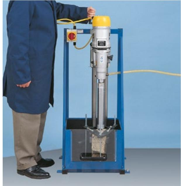
Cores may be cut from regular or irregular samples of rock or other material for end preparation prior to strength testing. Side guards and a drain tray provide protection against water spray and a sliding front allows access to the specimen clamp. The clamp provides maximum orientation for securing irregular block samples.
