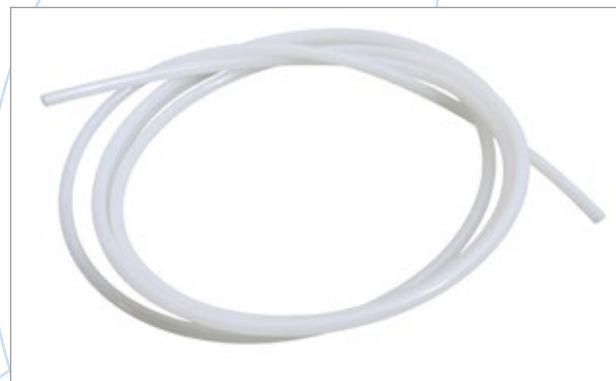
6 mm outside diameter x 4 mm inside diameter. For use up to a pressure of 3500 kPa. Priced per metre.
