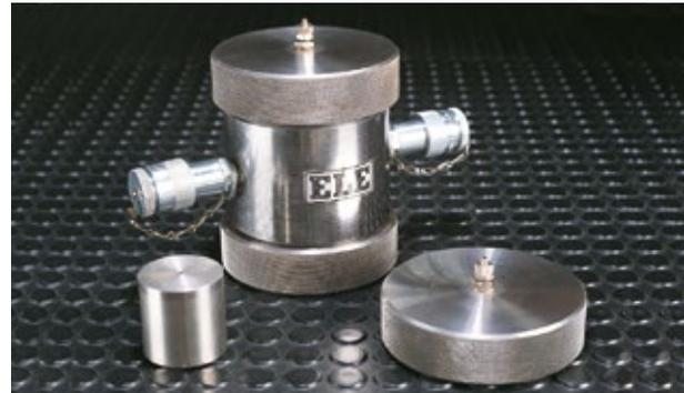
Permeability end caps used with ELE-Hoek Cells and constant pressure systems are a cost-effective solution suited to investigating the permeability of rock at high confining pressures in the laboratory. To collect and measure the water which permeates through the rock specimen, a suitable burette such as 25-4540 is recommended. Each permeability end cap incorporates a tubing connector which accepts standard 6 mm tubing, 26-1926, used to connect the cell to the pressure system and burette.
