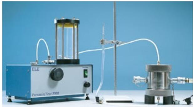
Permeability Test with Pressure Test 3500 Pressure System.
