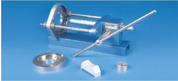
Extrudes the specimen from its jacket without the need to drain the confining fluid. Incorporates a rack and pinion mechanism mounted in a steel body, with adjustable back plate. Supplied with NX extruder adaptor set.
