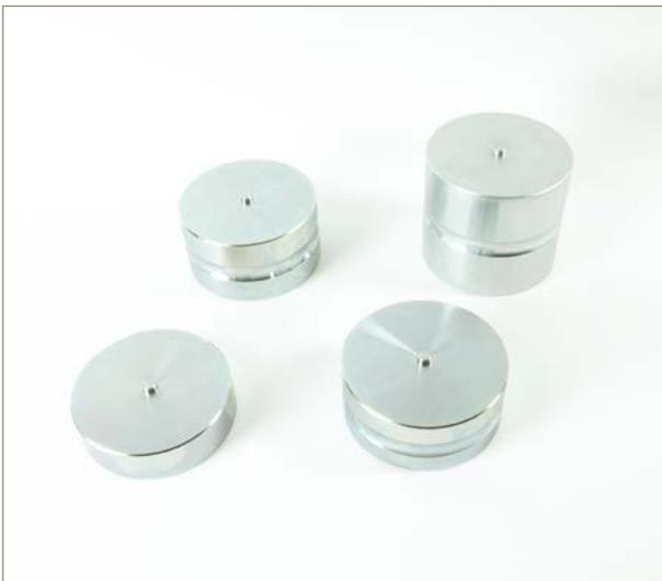
Accessory for testing samples 40 mm, 50 mm, 70.7 mm and 100 mm.
