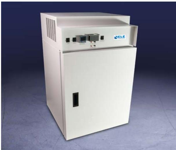
Prior to testing, prisms to be cured for a period of at least 24 hours at  $20^{\circ}\text{C} \pm 1^{\circ}\text{C}$ , 90% RH minimum. The prisms are then de-moulded and stored under water for the required curing time, usually 48 hours, 72 hours, 7 and 28 days.
